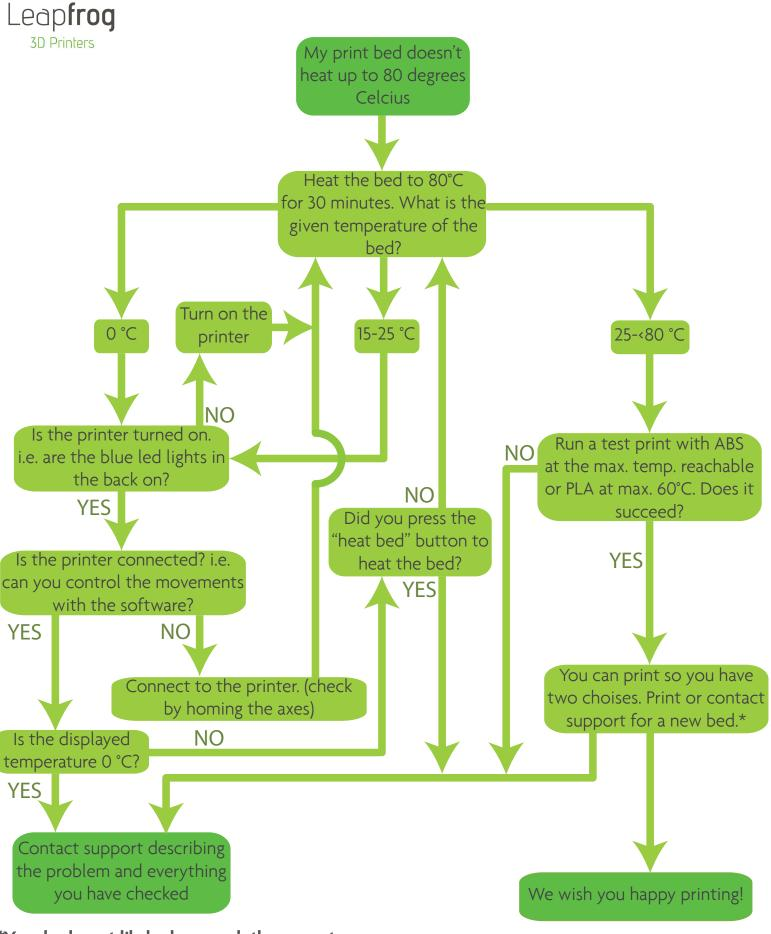
\*Your bed most likely does reach the correct temperature but due to insulation the thermistor displays a lower value for the temperature.
