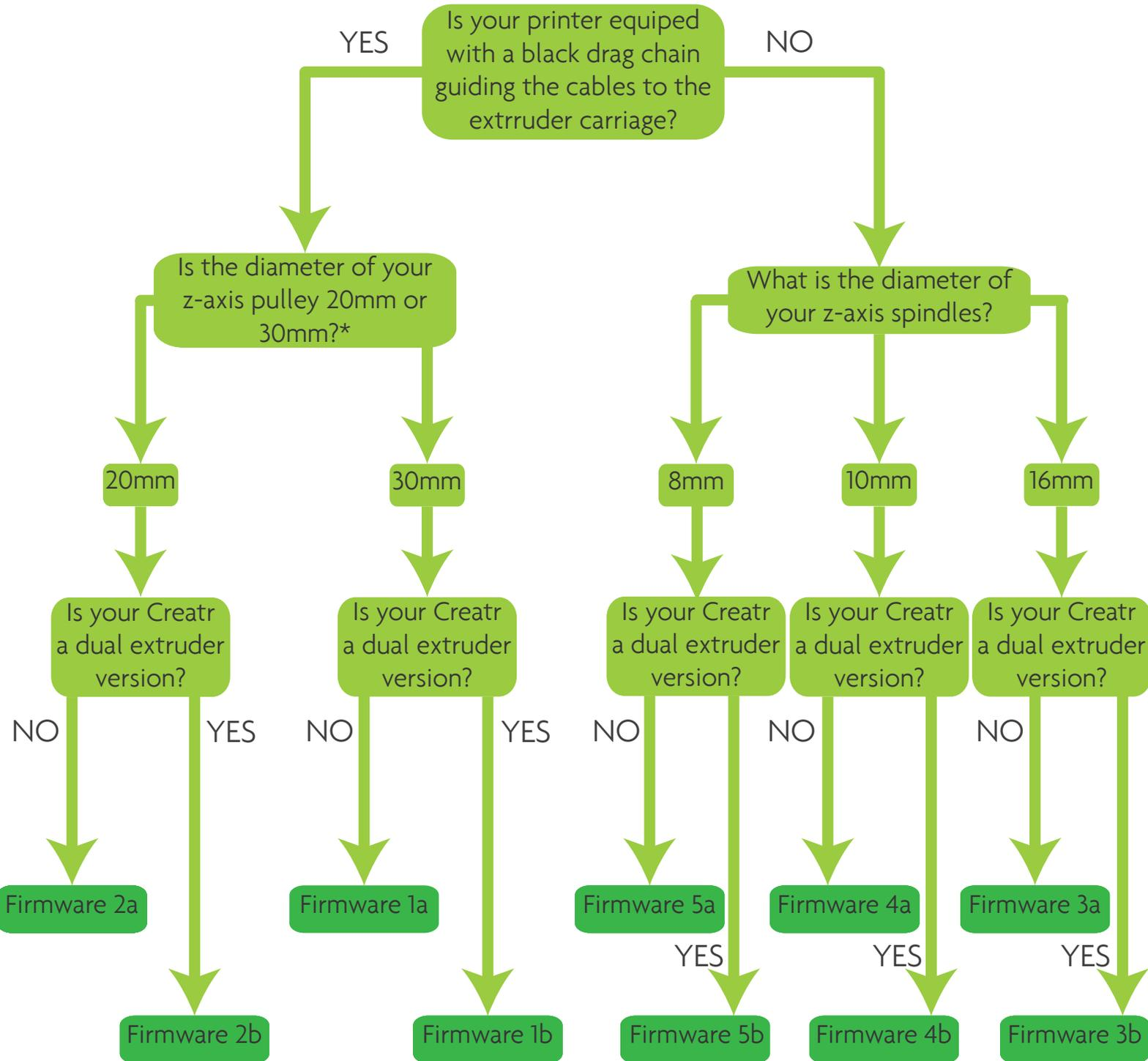
\*Par. 3.12 in the user manual explains how to check the size of your z-axis pulley
